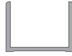
4101 Kapak Profili U connection profile 0,846 kg/m
